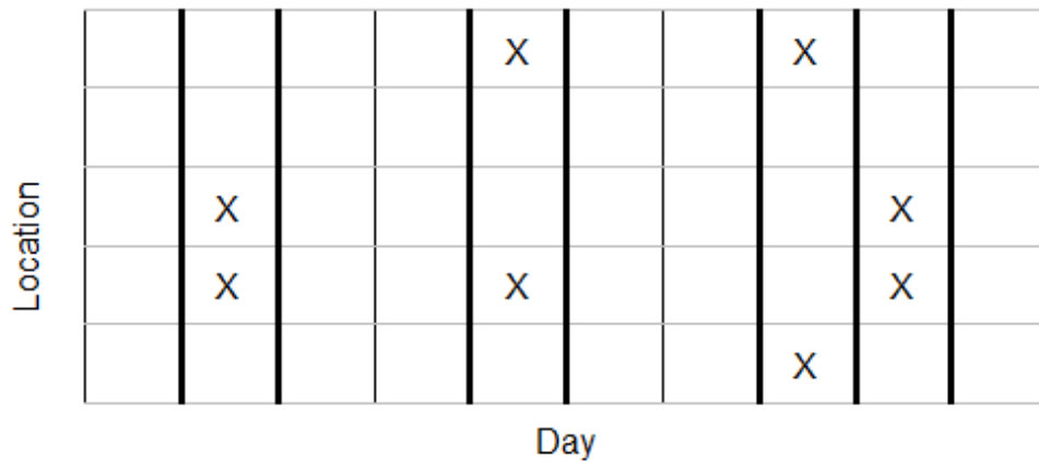
Figure 3. A two-stage cluster sample. At the first stage, 4 clusters (days) are selected. These are shown by the heavy lines. At the second stage, two locations are selected from each cluster (day).
